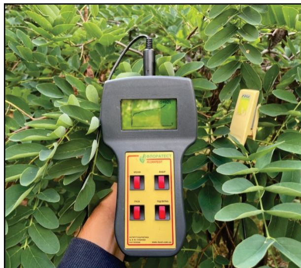
Fig. 1. Instrumental support for the field experiment: portable fluorometer “Floratest”
