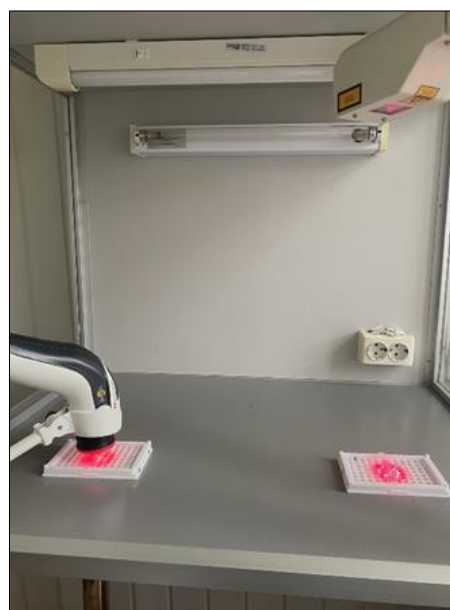
Fig. 1. Irradiation of microbial biofilm by PILER (on the left) and laser radiation (on the right)
