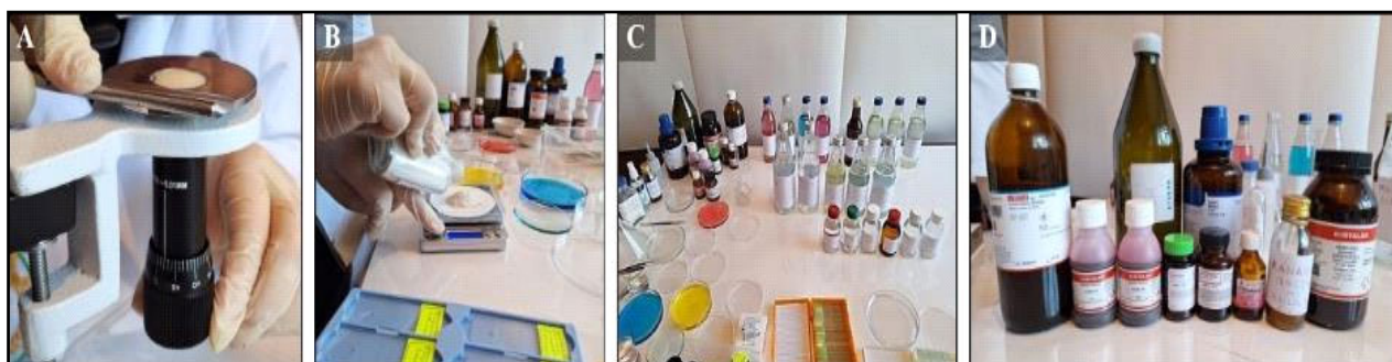
Fig. 2. The hand microtome (A) used for obtaining sections from plant samples, the process of preparing the sections (B, C), and the reagents (D) used
