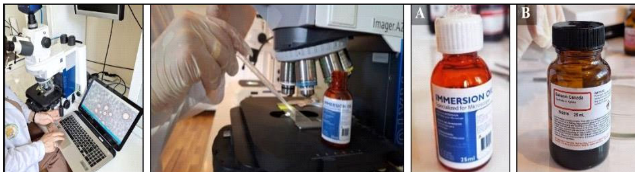
Fig. 3. Conducting an anatomical analysis using Axio imager A2 optical microscope model, utilizing immersion oil (A) in this analysis, and employing Canada balsam (B) in the preparation of specimens
