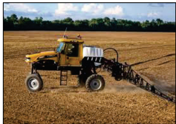
Fig. 2. Application of the biological destructor solution to the stubble using the self-propelled field sprayer SPRA-COUCPE
