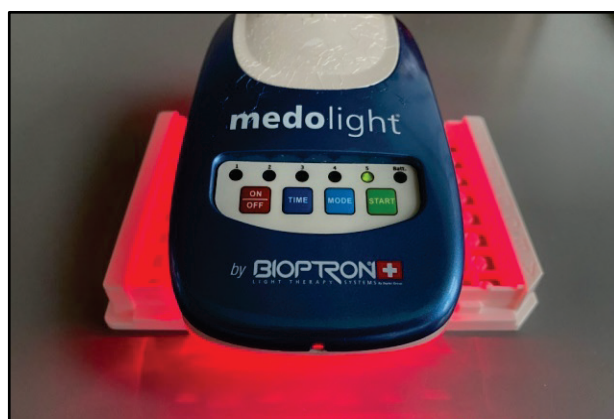
Fig. 1. Irradiation of microbial biofilm by LED light generated by Medolight Red device (Zepter, Switzerland, 2017)
